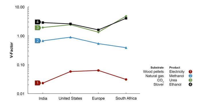
Figure 2. The V-factor for a manufacturing process varies with geography. For each process, the fractional yield is usually constant with respect to location. However, the values of the reactants and/or products vary from region to region since pricing is heavily influenced by regional factors that control demand and supply. The raw data employed for the calculation of the V-factors is presented in Table S3 in the appendix.
