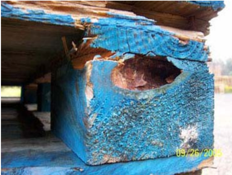
Figure 4e. "Barky" defect in pallet deckboard.
