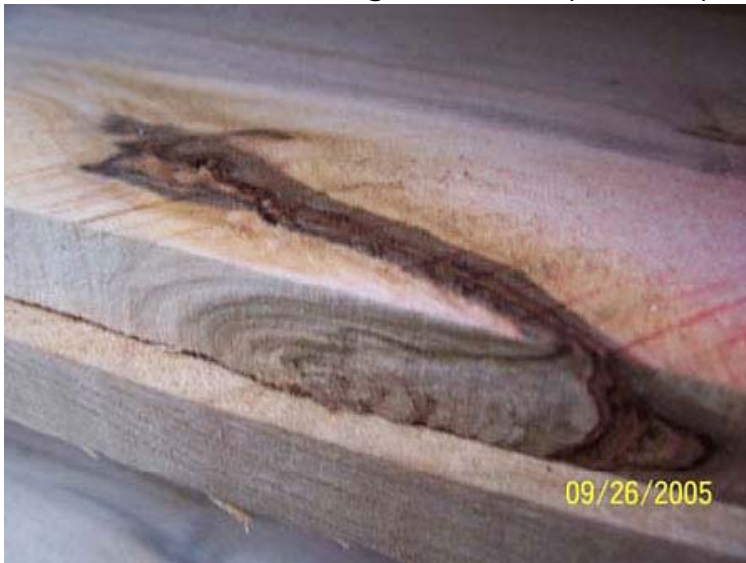
Figure 4c. Bark pocket in pallet deckboard.
