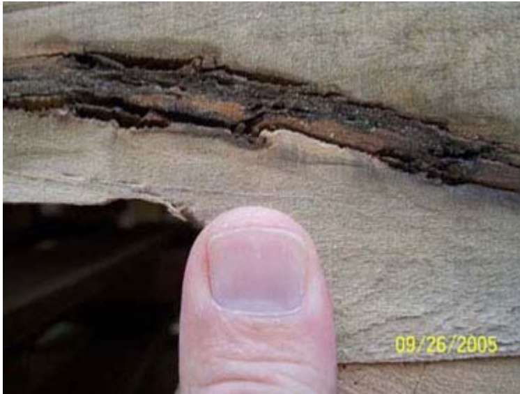
Figure 4c. Bark pocket in pallet deckboard.
