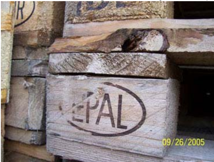
Figure 4e. "Barky" defect in pallet deckboard.
